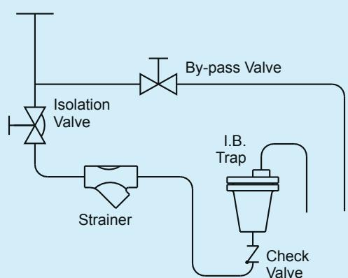
Fig. 1 shows a simple arrangement of trap module in open loop. This consists of the end flange, Isolation valve, a trap and the by-pass valve.
