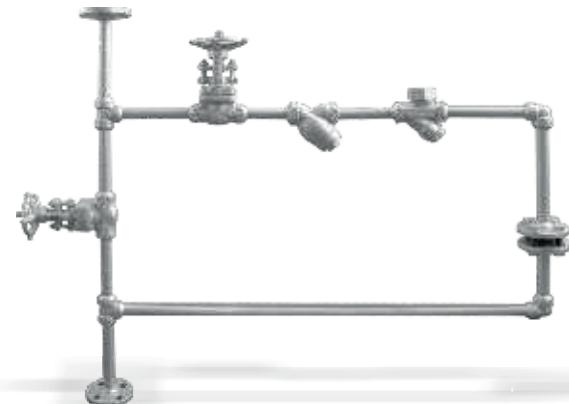
Inlet and outlet isolation valves are provided to facilitate removal of the steam trap and its accessories for maintenance.
