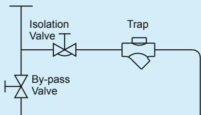
Fig. 2 Liquid drain trap module with balancing line
