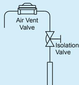
Fig. 4 Trap module in closed loop
