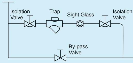
Fig. 5 Inverted Bucket trap module in open loop
